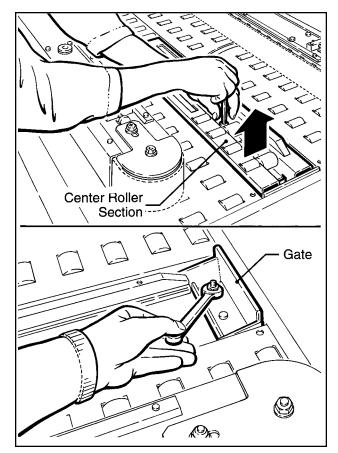
Figure 5-4 – Gate Stroke Setting
